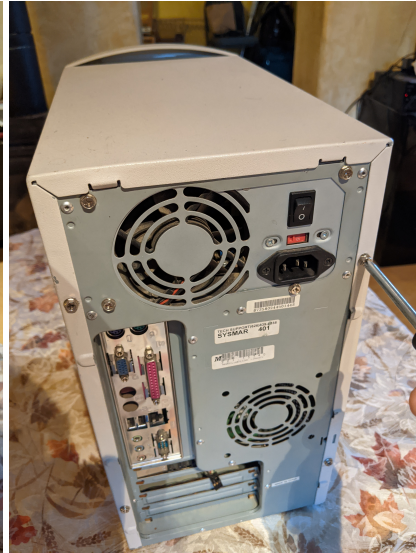
(b) The back - note opening screws and connectors.
